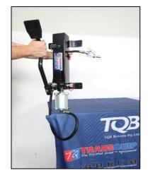
2. Hold the pump on the edge of the bench and operate the manual pump pedal until the attached ram has extended to over half of its stroke.
